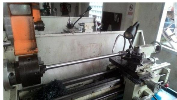
**Gambar 5.** Proses pengupasan logam
