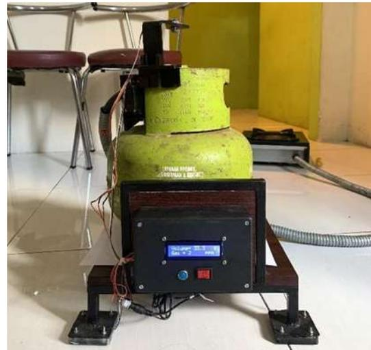
Gambar 5. Alat pendeteksi kebocoran gas
