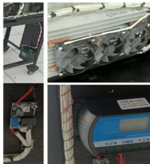
Gambar 10. Akumulator, *step up* tegangan, *charger* akumulator, dan kipas pendingin.
