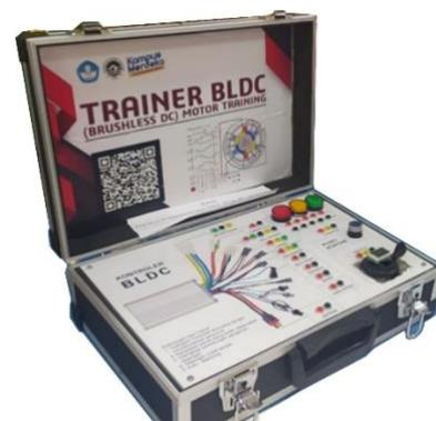
Gambar 3. Media Sistem Kerja Motor BLDC
