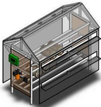
Figure 1. Design of automatic mushroom house
