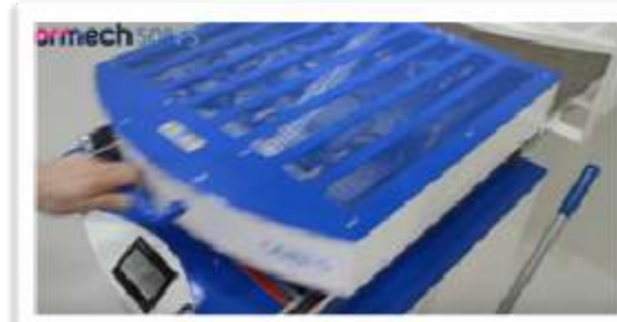
Figure 14. Steps in the vacuum forming process: Acrylic vinyl heating below. Documentation: formech.com, 2017.
