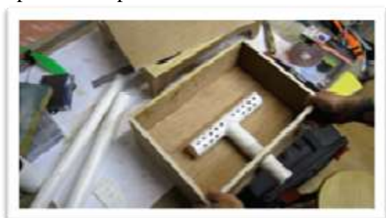
Figure 17. Bottom box that has been pipe fitted as a lane to suck air using a vacuum cleaner tool commonly used in many homes. Documentation: Roboforcex2000, 2017 (10)
