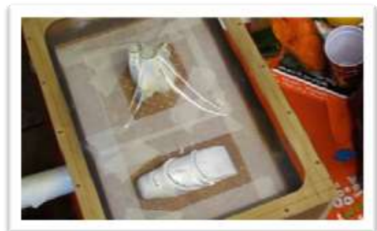
Figure 21. The heated plastic sheet is placed over the master object then sucked.
