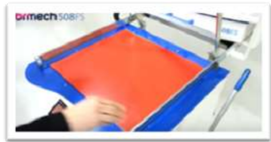
Figure 13. Steps in the vacuum forming process: Acrylic vinyl prepared above. Documentation: formech.com, 2017.
