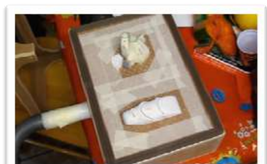
Figure 21. The master object to be duplicated is placed on the evaporator board, the unwanted hole is covered with the lackban so that the suction area is focused on the master object.
